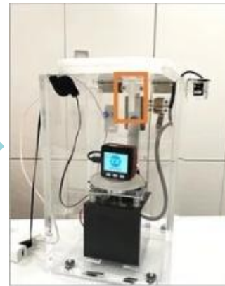
A soft absorber allows the table to lower gently
